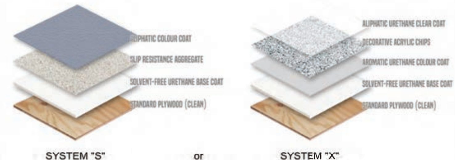
2 A2 DETAIL OF COVERED DECK WATERPROOF FLOOR MEMBRANE NOT TO SCALE
